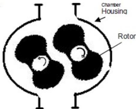
Because there is no friction between the moving parts, the Root Blower allows high-speed rotation for giving out high flow-rates.
